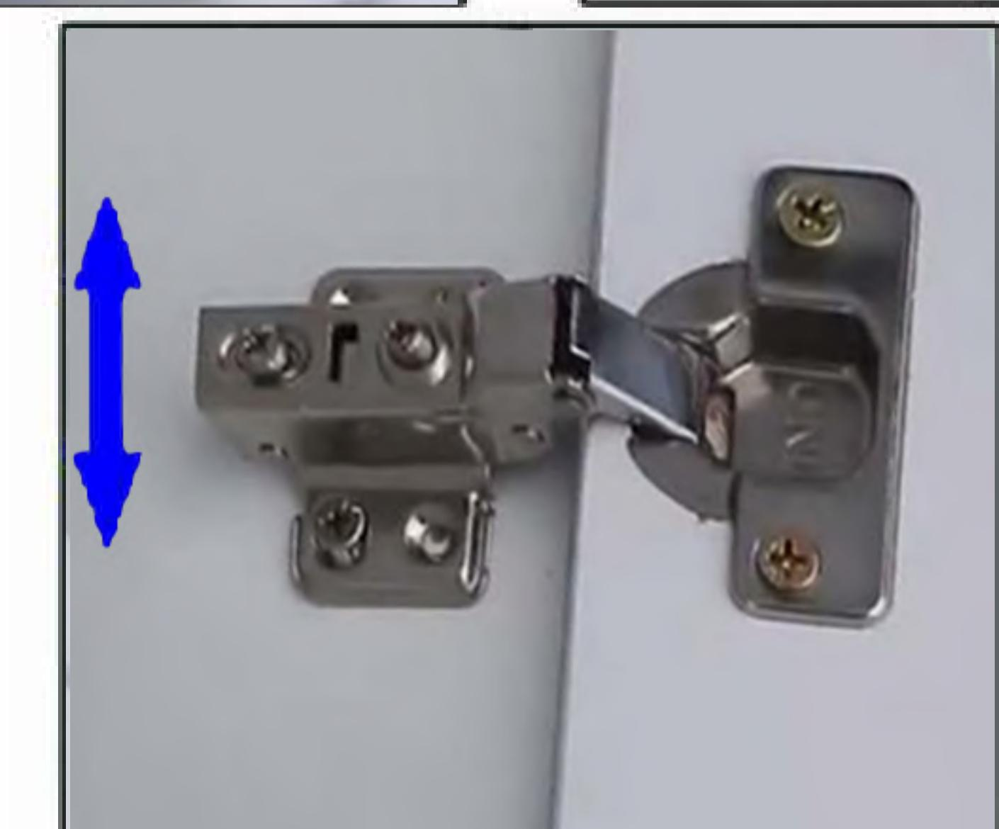
As shown in the figure, loosen the screw that the screwdriver points to, push the lower door panel and hinge upward, and then tighten the screw. Push the upper door panel and hinge downward, and then tighten the screw.
