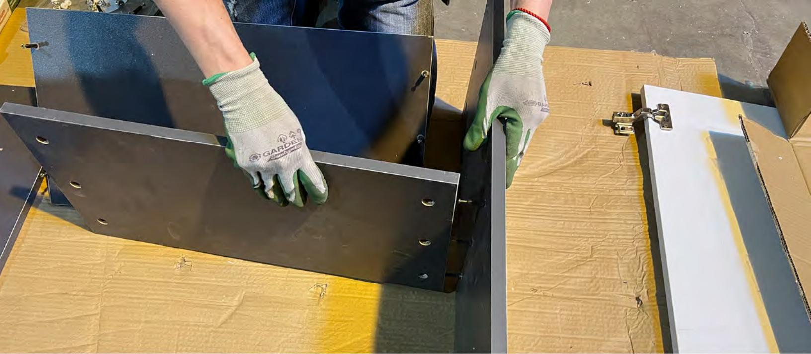
When connecting the panels, make sure the side with the small pre-drilled holes is facing down.
