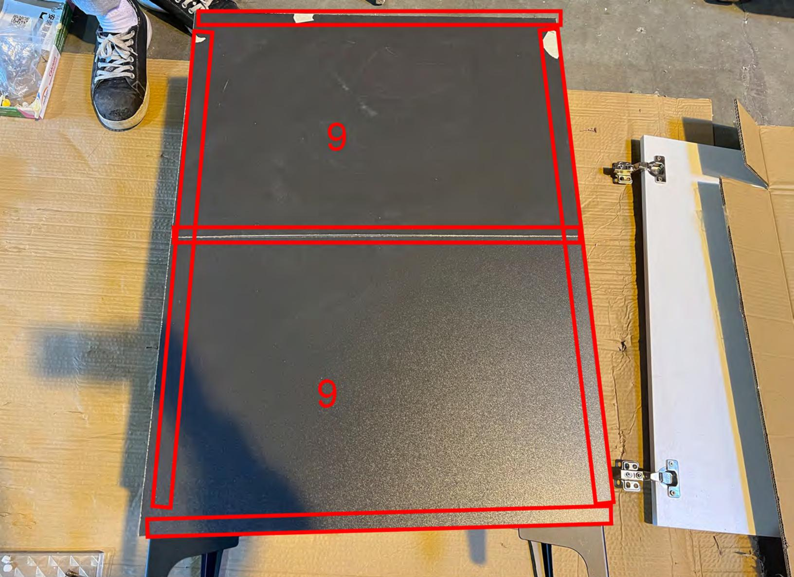
Place 9 (the back panel) in the correct position, fully covering the back side of the cabinet. Make sure to leave enough space along the edges for proper fastening. 9 x 2 should be installed using the same procedure.
