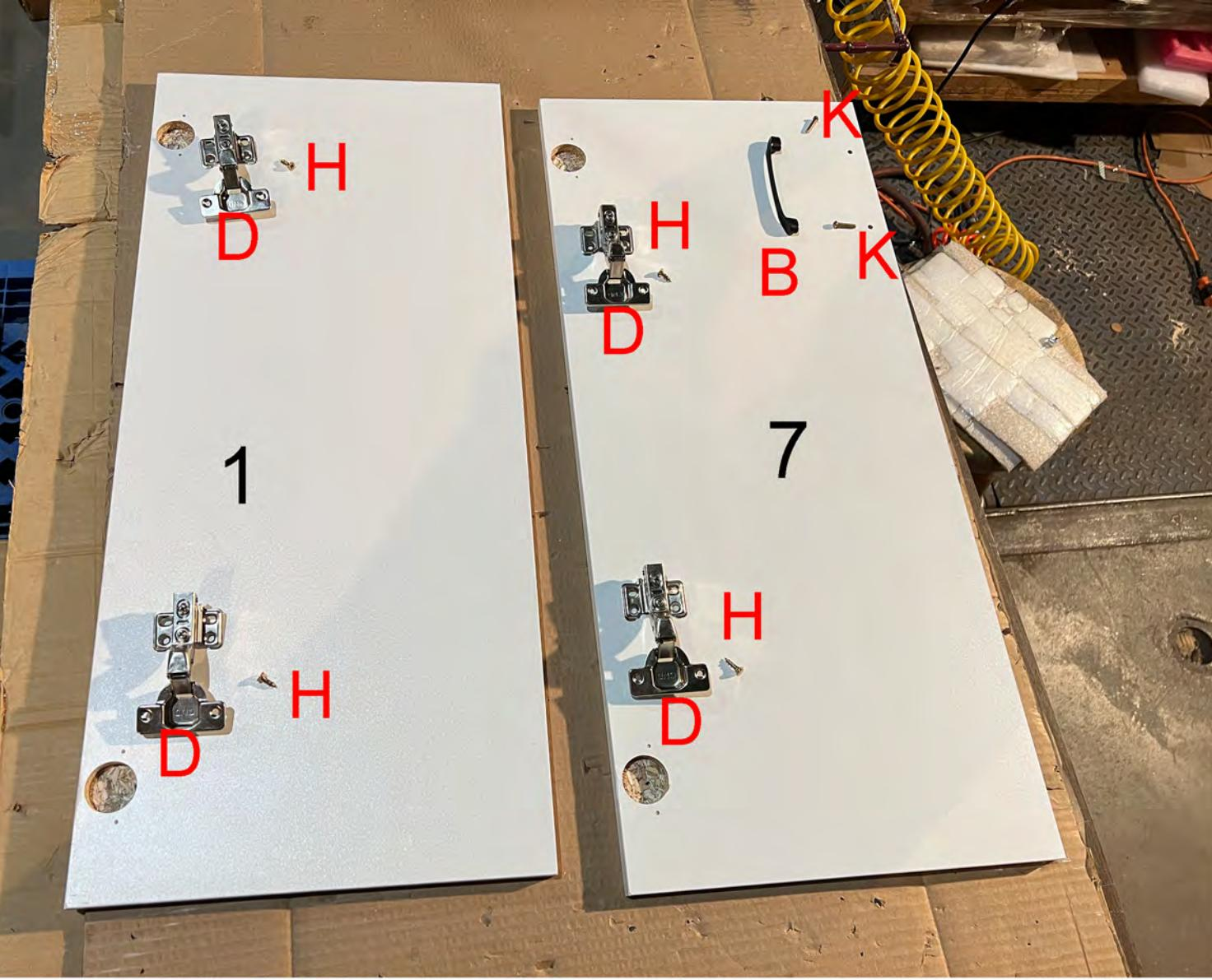
Panels 7, attach B using K. Install B on the outer-facing side.
