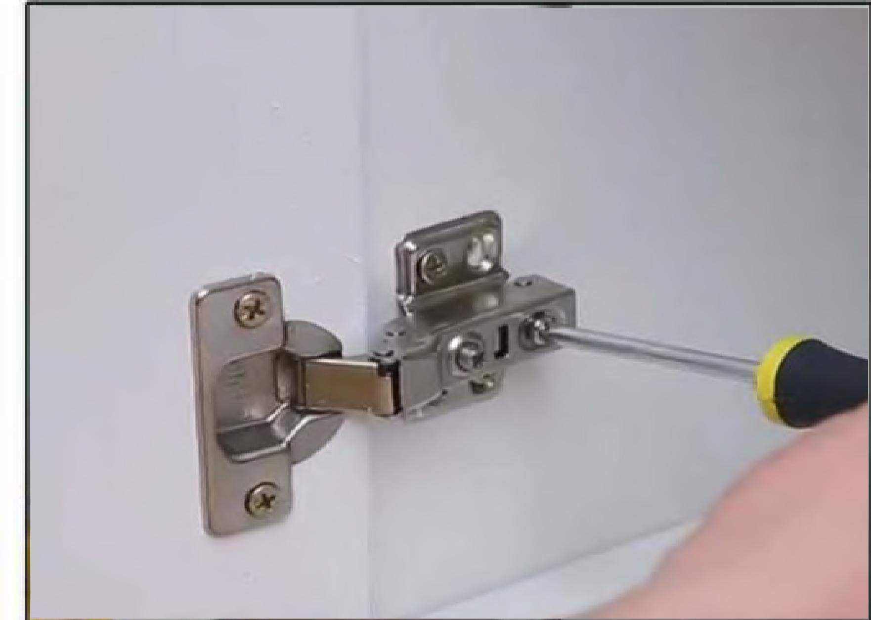
As shown in the figure, loosen the screw that the screwdriver points to, push the door panel in or pull it out, and then tighten it to solve the above problem.
