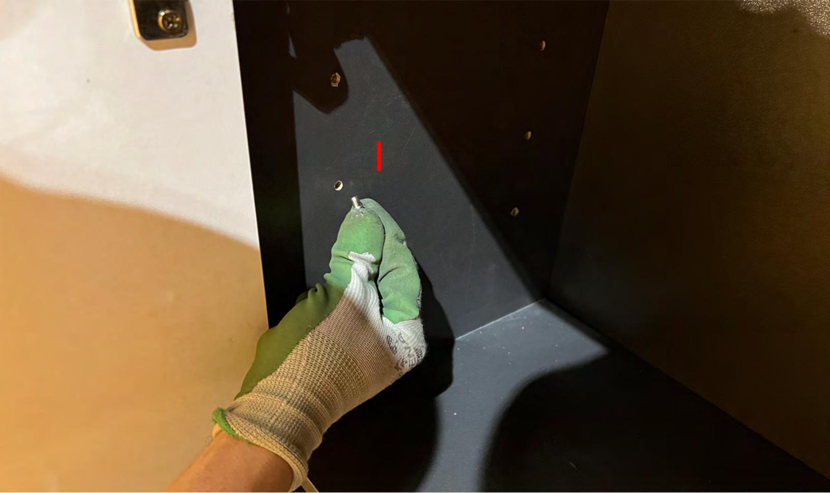
Install part 8 as needed. Insert part I into the matching pre-drilled hole on the appropriate side panel.
