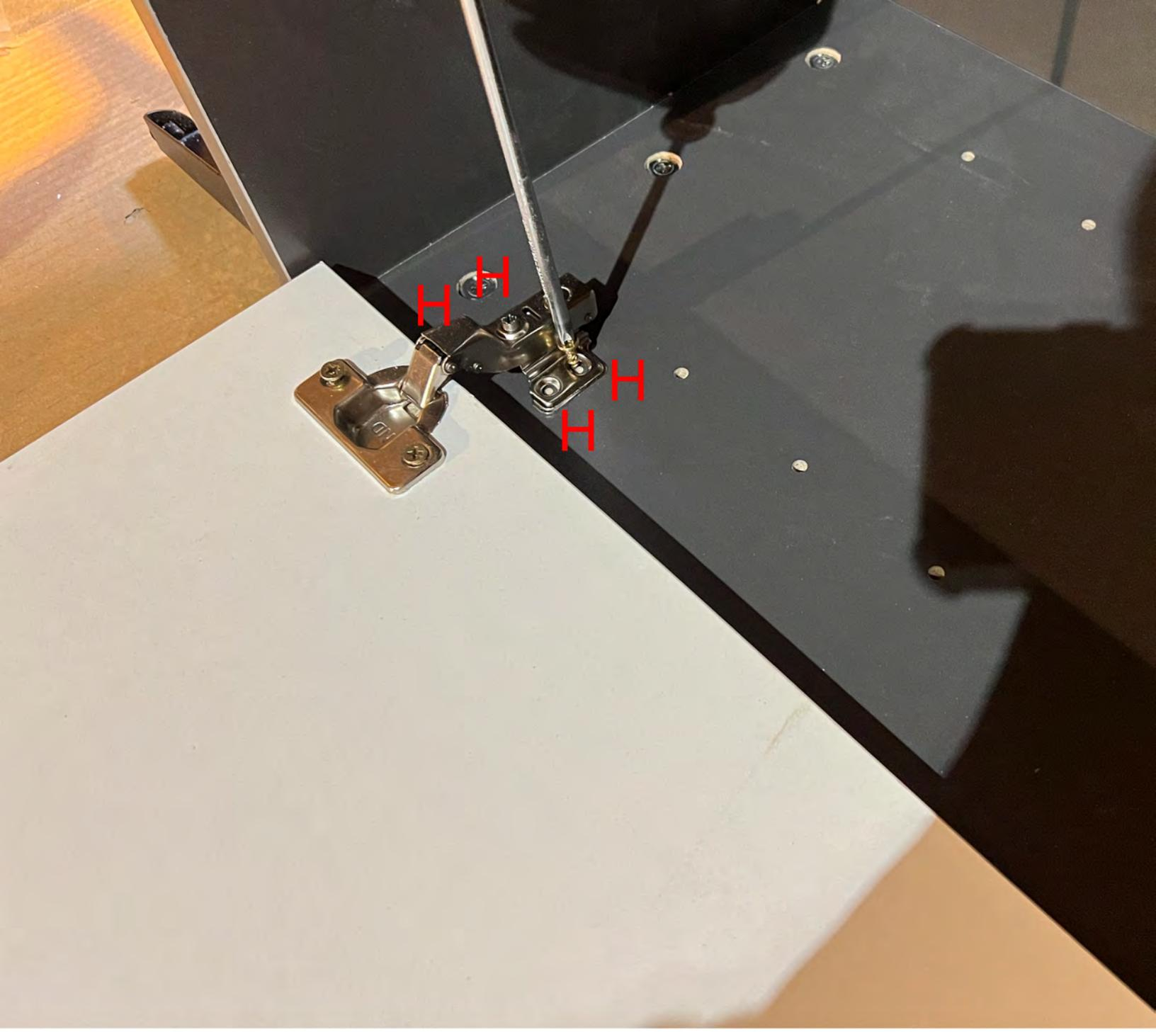
Line up the four holes on the hinge with the nearby holes on the side panel and attach it using H. You can adjust the door's height slightly—aim for even spacing rather than following the pre-drilled holes exactly.
