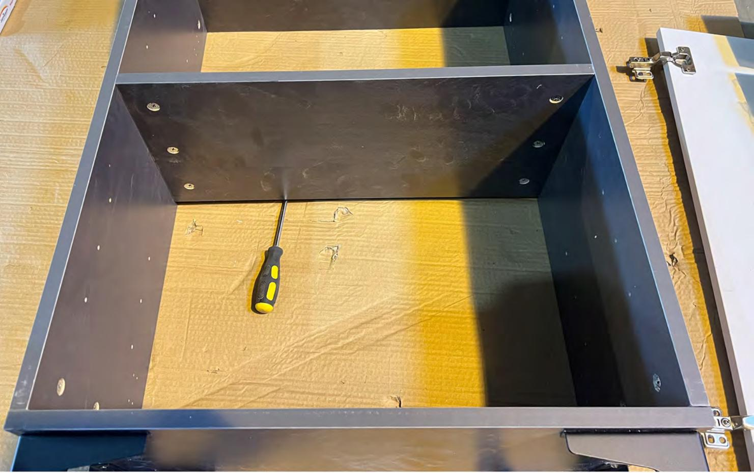
Inspect the bottom for gaps. If none are visible, verify that all panels are oriented correctly.
