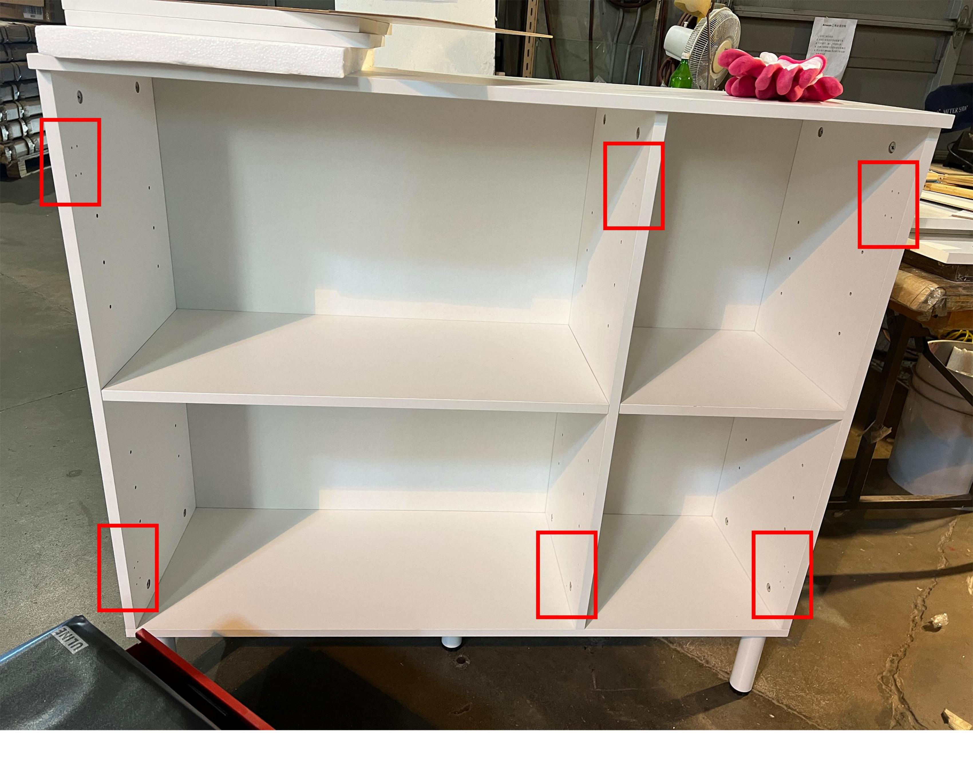
You may first stand the cabinet upright. Ensure that all groups of 4 positioning holes are facing forward to confirm proper orientation.
