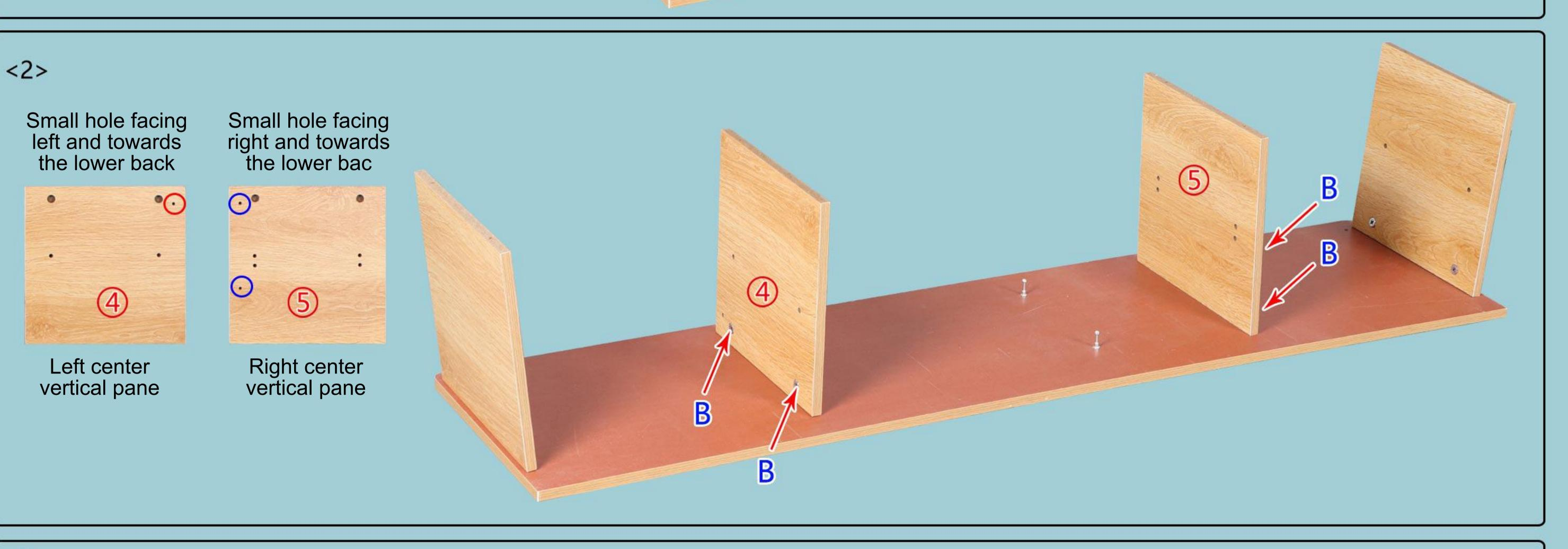
Lock the board with an eccentric bolt by rotating it clockwise
