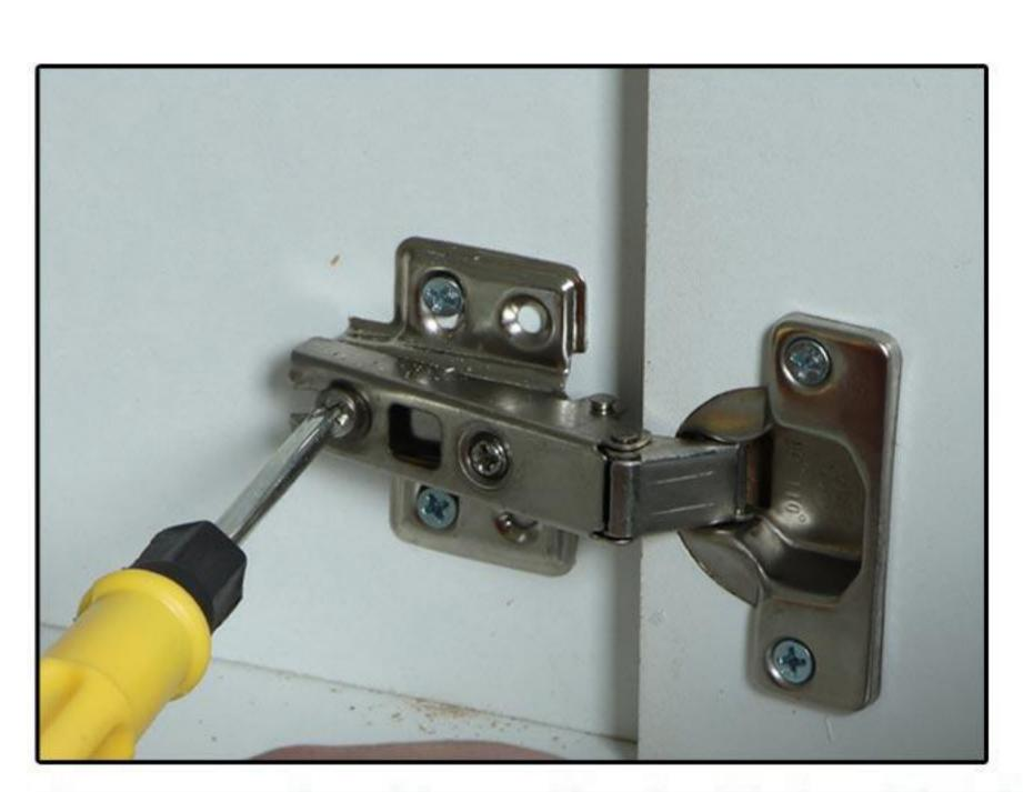
As shown in the picture, loosen the screw pointed by the screwdriver, push the door panel in or pull it out, and then
