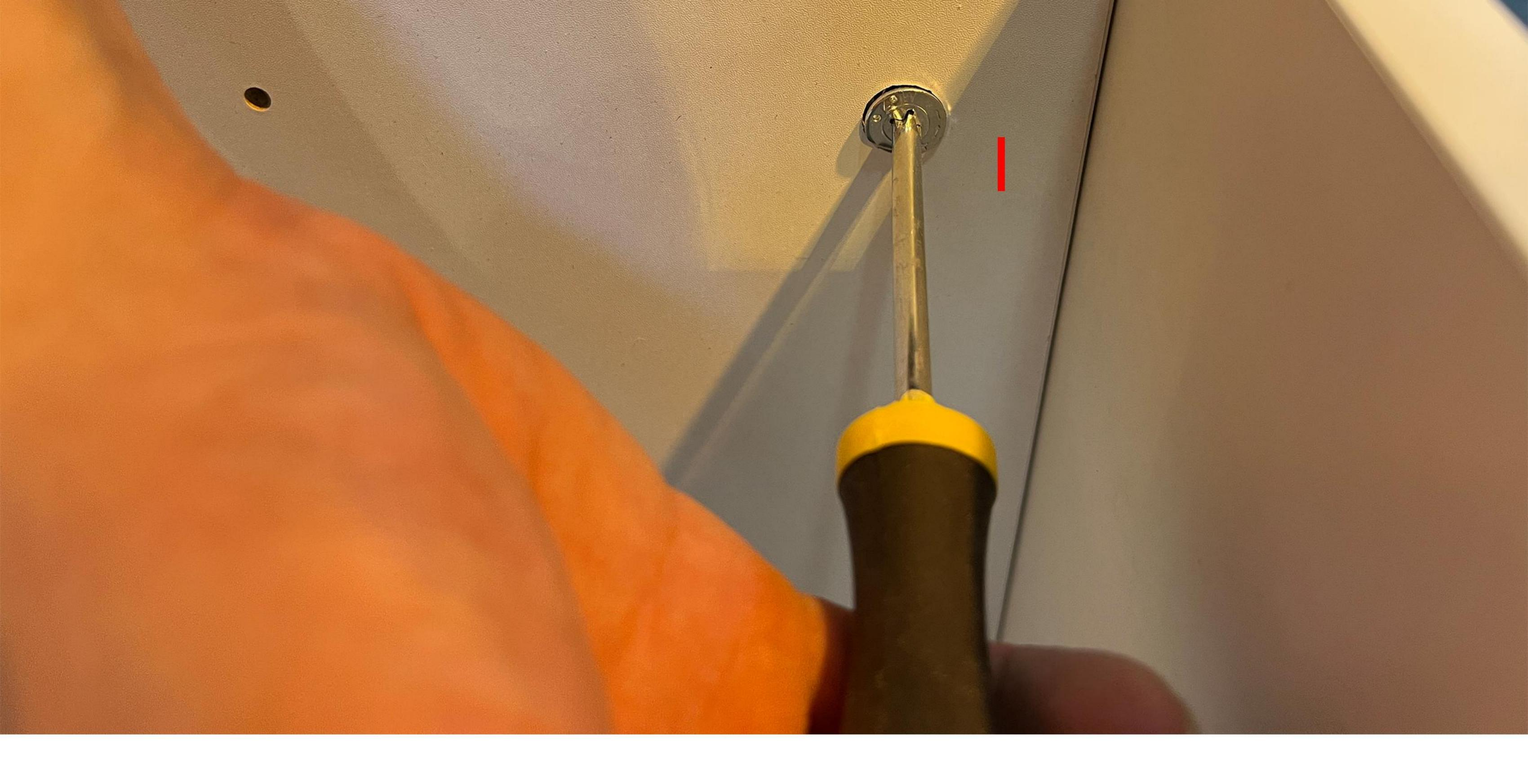
Secure part I into the large pre-drilled holes. Refer to the "Instructions for Using Eccentric Bolts" for detailed guidance.
